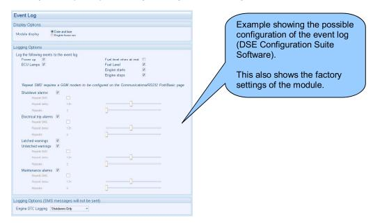
When the event log is full, any subsequent event overwrites the oldest entry. Hence, the event log always contains the most recent events. The module logs the event type, along with the date and time (or engine running hours if configured to do so).
