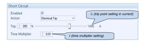
The effect of a short circuit on the generator is that the alternator stator and rotor begin to overheat; the aim of the *IDMT alarm* is to prevent the stator and rotor being overload (heated) too much. The amount of time that the alternator can be safely overloaded is governed by how high the short circuit condition is.
